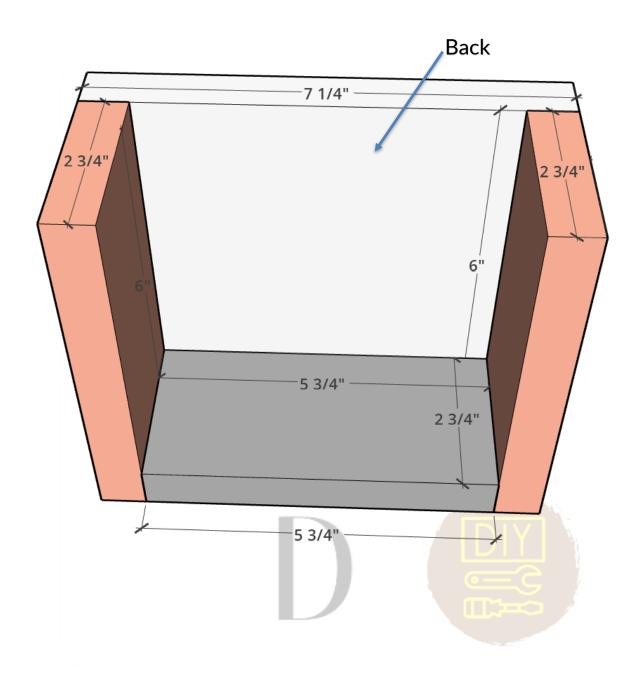
**Step 4**Attach the front right piece using wood glue and brad nails. Three nails on the side and one or two at the bottom should be enough.
