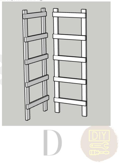
**Step 4**Secure the upper and lower pieces to assemble the leg and form the frame.
